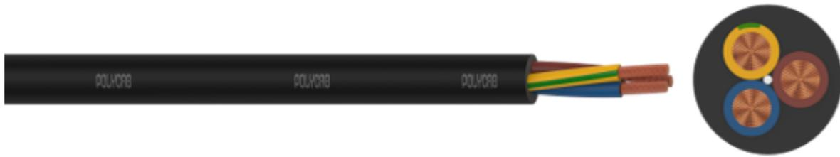
These are flexible fire performance cable with low smoke zero halogen thermoplastic insulation for connection of domestic appliances to the fixed supply. This covers low voltage energy cable confirms the construction and performance of thermoplastic insulated cable of voltage rating up to and including 300/500 V as per BS EN 50525-3-11. These cables emit low smoke and corrosive gases when exposed to fire. These are intended for the connection of domestic appliances to the fixed supply.
