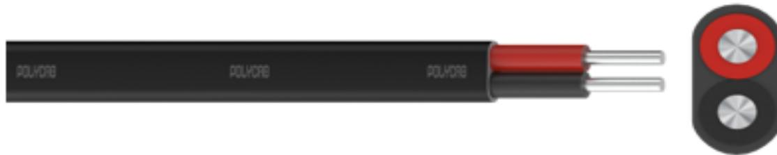
These are low voltage cable of 1100 V grade, PVC insulated, and sheathed Aluminium flat cable is suitable to use for industries, buildings, and complexes where armouring protection is not required. These cables are available with operating temperature rating of 70°C.
